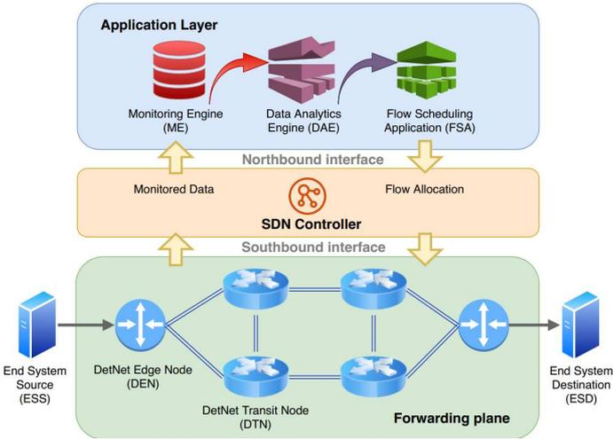
Fig. 1: SDN-like DetNet network architecture considered in this work.
