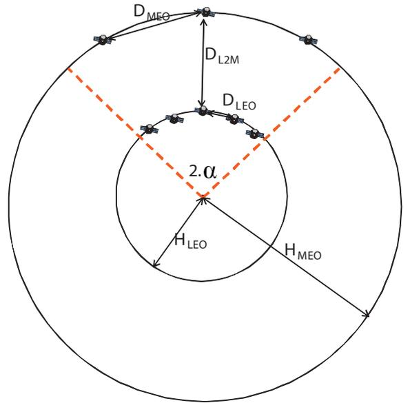
Fig. 2. A simplified model of a multi-layer LEO/MEO satellites network.
