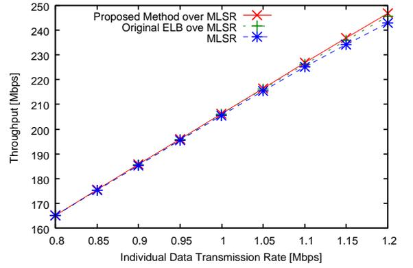
Fig. 4. Total throughput for different individual sending rates.
