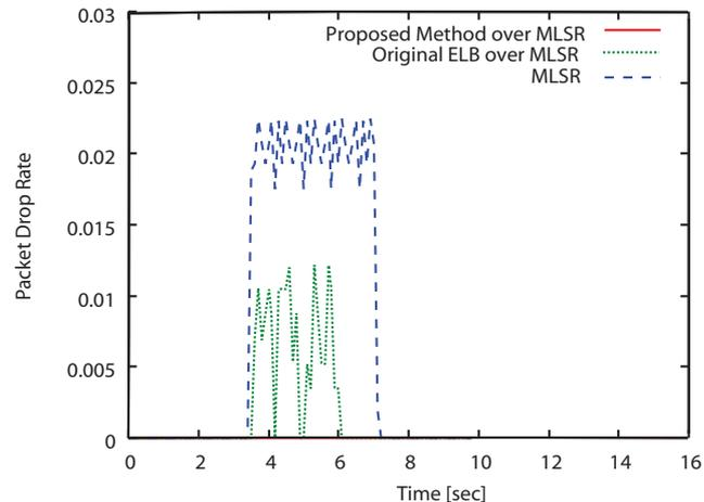
Fig. 7. Packet drop rates at a particular satellite over time.
