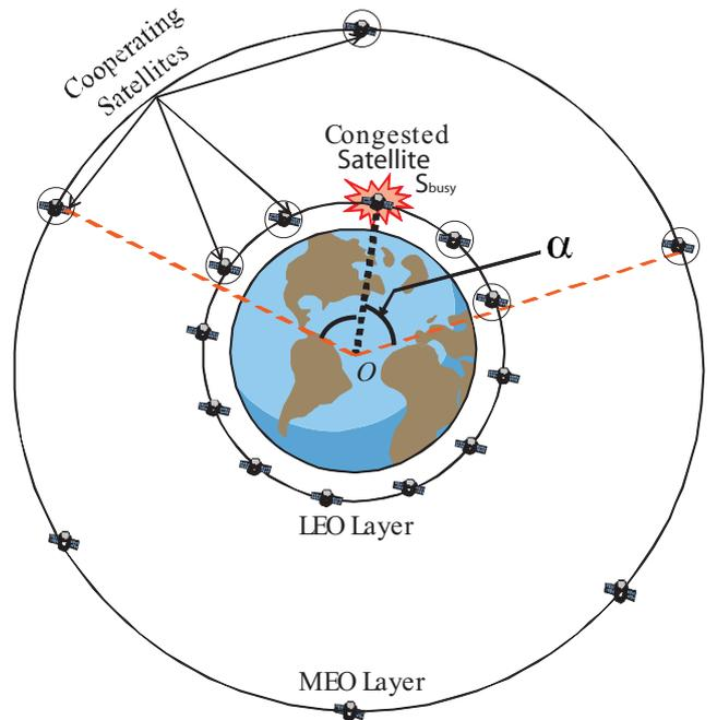
Fig. 1. Range of BSAs exchange based on the angle  $\alpha$ .
