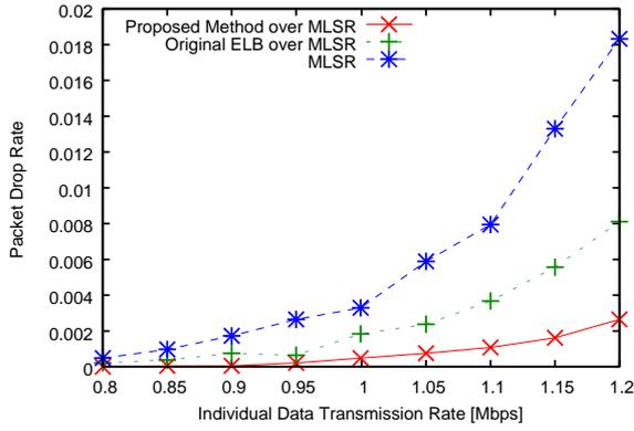
Fig. 3. Packet drops for different individual sending rates.
