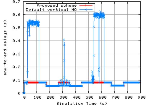
Fig. 6. Instantaneous end-to-end delays during the simulation time.
