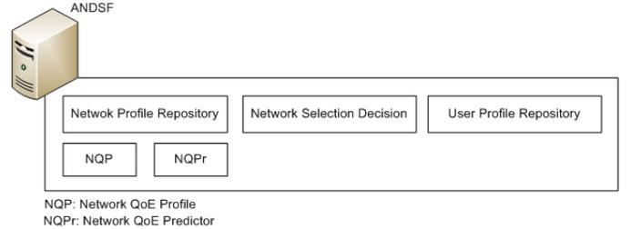
Fig. 2. Proposed additional components to ANDSF or alike node.
