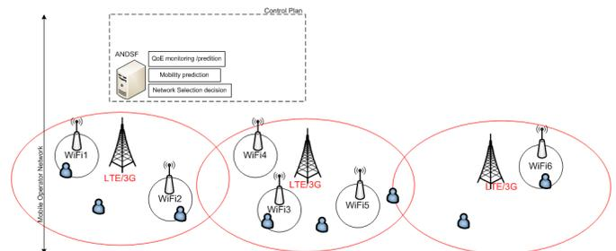
Fig. 1. Envisioned mobile network architecture.
