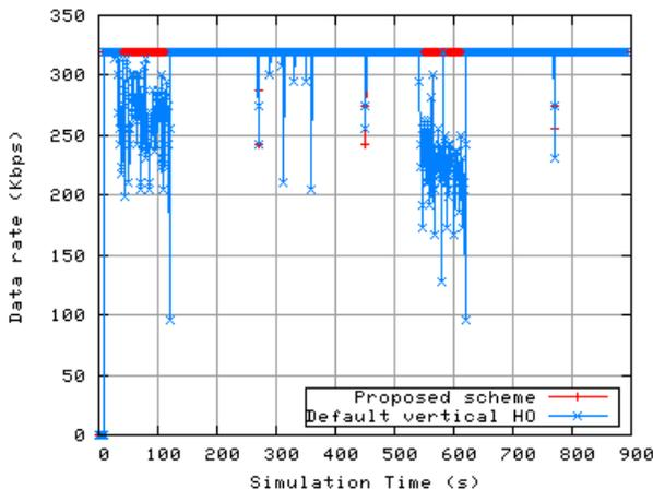
Fig. 5. Instantaneous data download rate during the simulation time.
