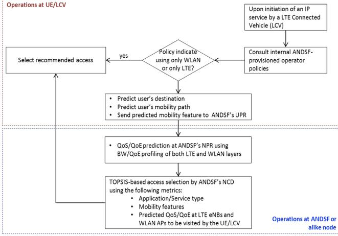
Fig. 3. Proposed wireless access steering mechanism for vehicles connected to LTE (or to other suitable mobile access technology).
