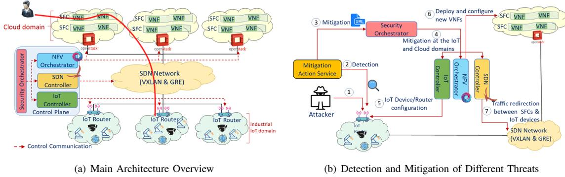
Fig. 1: Envisioned System: Architecture and Security Enablers
