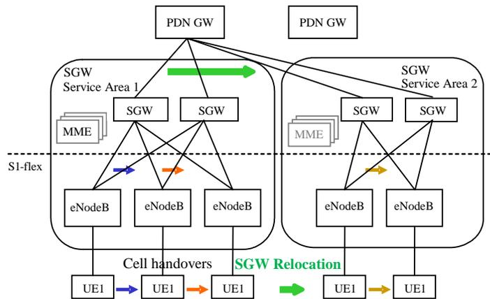
**Figure 1. SGW service or pool areas – with fix/hard SGW relocation borders at service or pool area boundaries.**
