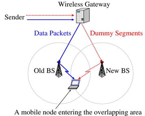
Fig. 1. Upon a handoff occurrence, two connections are simultaneously set between the mobile node and the sender upon its entrance to the cell overlapping area: One through the old BS and the other through the BS of the new network cell.
