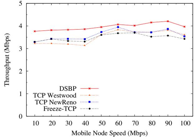
(b) Case II: Handoff from a high bandwidth cell (6 Mbps) to a low bandwidth cell (1 Mbps)
