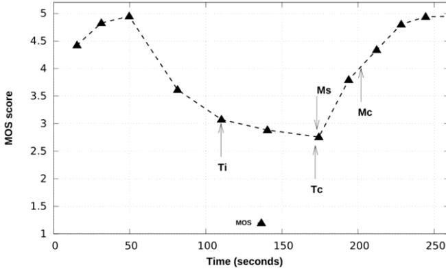
Fig. 5. MOS vs Time (full functionality). (*Ti*: transcoding container initiated; *Tc*: transcoding completed; *Ms*: mixing started; *Mc*: mixing completed).
