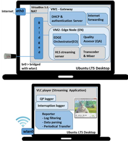
Fig. 3. Test-bed setup.
