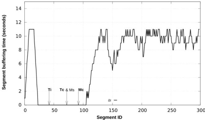
Fig. 6. Segment buffering time ( $\Delta t$ ) vs Segment ID. (*Ti*: transcoding container initiated; *Tc*: transcoding completed; *Ms*: mixing started; *Mc*: mixing completed; when Segment buffering time = ‘0’, corresponding segments are not downloaded in advance).
