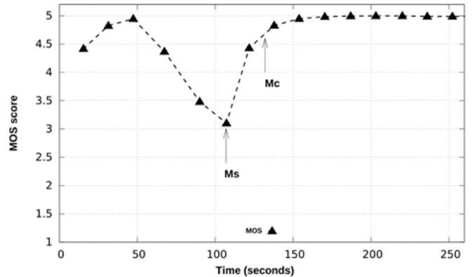
Fig. 4. MOS vs Time (with pre-transcoded media files). (Ms: mixing start time; Mc: mixing completion time).
