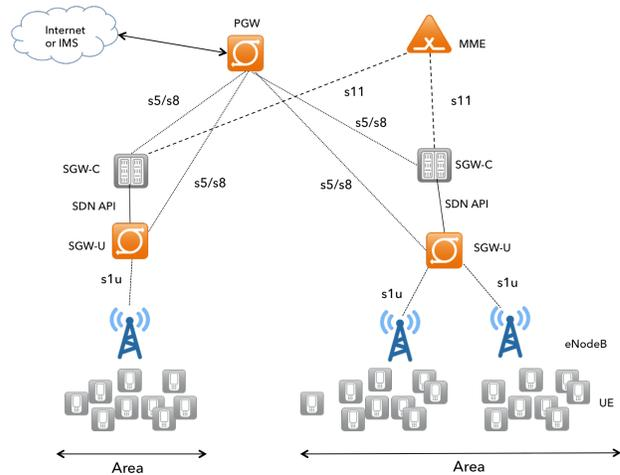
Fig. 1. Envisioned SDN-based mobile network architecture
