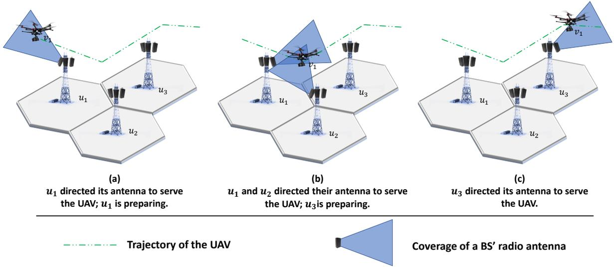
Fig. 2: Illustration of AMC principle: BSs dynamically adjust the direction of their radio antennas so to cover the trajectory of the UAV.
