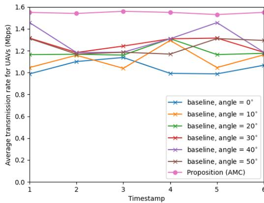
Fig. 5: Comparison of the proposed approach against baseline solutions (fixed angles of the BSs' radio antennas).
