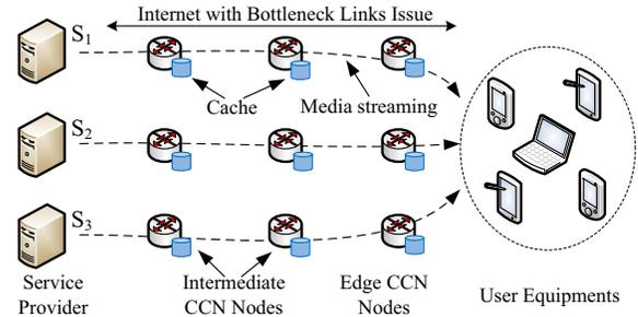
Fig. 1. Example for multi-source transport of media and in-network caching.
