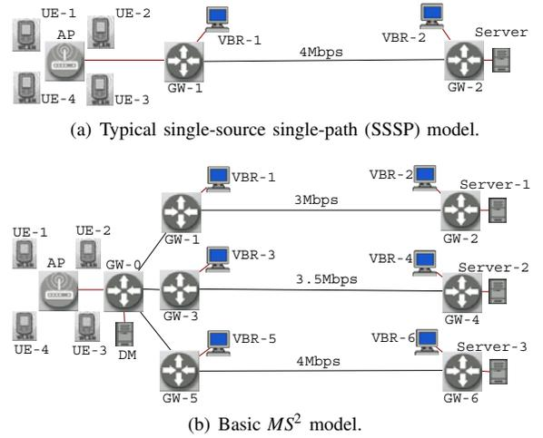
Fig. 2. Mobile multimedia streaming via a single access point: single-source single-path streaming vs.  $MS^2$ .
