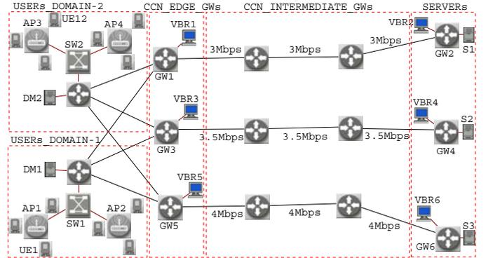
Fig. 5. MM3C model with edge GWs caching (GW-1, GW-3 and GW-5).
