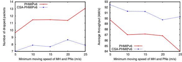
(a) Packet drops vs. moving speeds of the mobile nodes for PHMIPv6 and CSA-PHMIPv6 schemes. (b) Average throughput vs. moving speeds of the mobile nodes for PHMIPv6 and CSA-PHMIPv6 schemes.
