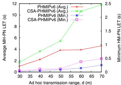
Fig. 9. PN's LET values over different transmission ranges.
