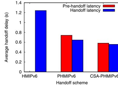
Fig. 5. Handoff delay for the three considered schemes.
