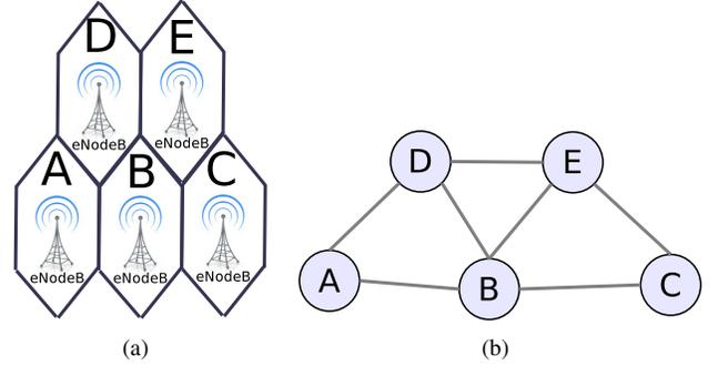
Fig. 1: An example illustrating how to construct neighboring graphs  $G$  from an LTE network.
