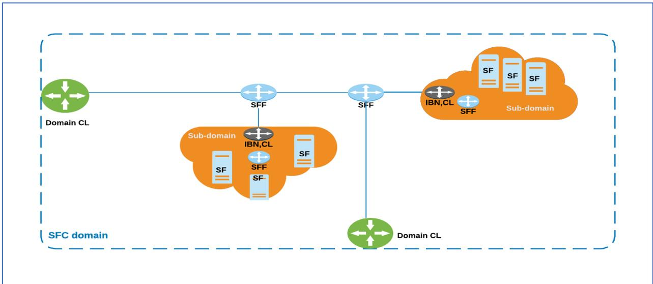
Figure 3: Architecture of Hierarchical SFC, where the SFC sub-domains are seen as single SFs to the higher SFC domain.
