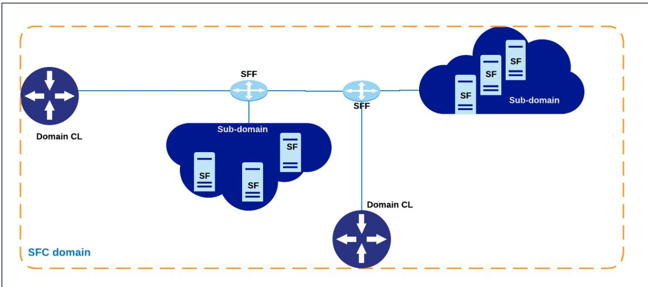
Figure 2: An example of Service Function Chaining Architecture, where the SFs in the sub-domain are visible to the SFC domain’s SFFs.
