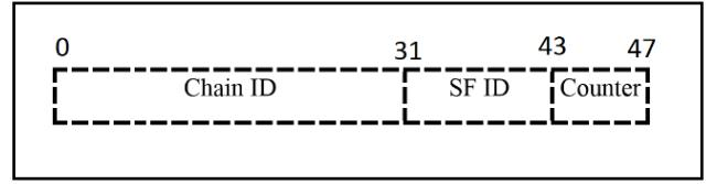
Figure 1: format of the SFC Compact header
