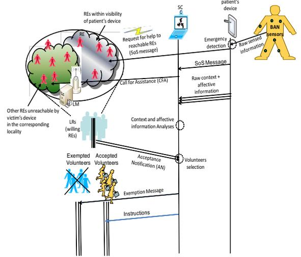
Fig. 1. The messages exchanged between different entities in PEACH framework upon detection of an emergency event.
