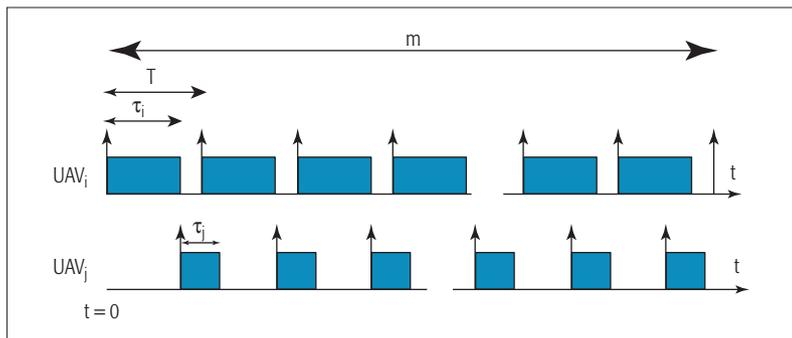
Figure 2. A snapshot of the activity schedule for two autonomous UAVs.
