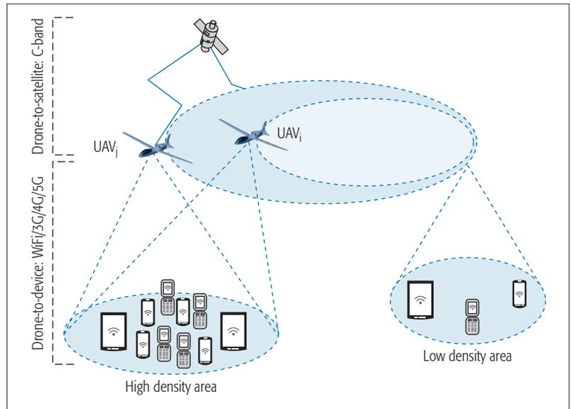
Figure 1. Drone small cells for coverage expansion.
