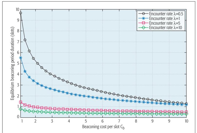
Figure 5. Equilibrium beaoning duration as a function of the beaoning cost (energy consumption) under different  $\lambda$ .
