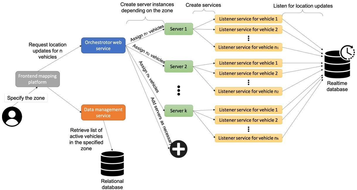
Fig. 5: A solution for ensuring short latency in vehicle location update and tracking regardless the number of connected vehicles.
