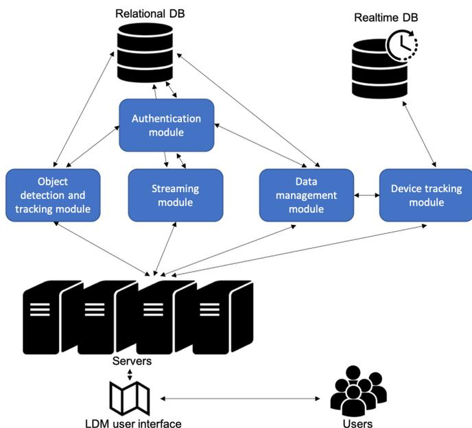
Fig. 1: Overview of the envisioned system architecture.
