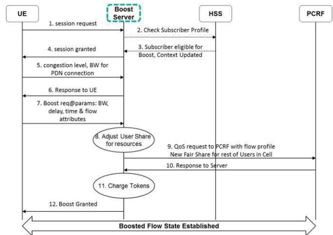
Fig.2: Process for requesting a Service Boost in LTE
