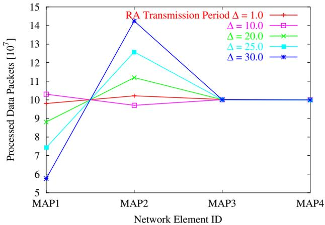
Fig. 4. Number of data packets processed at each MAP for different values of  $\Delta$ .
