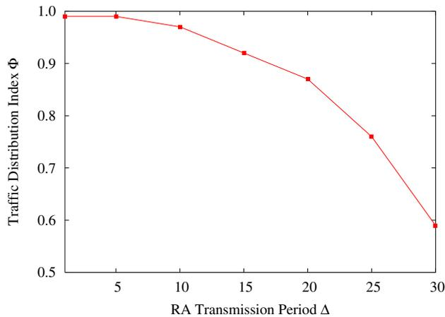
Fig. 5. Traffic distribution index  $\Phi$  for different values of  $\Delta$ .
