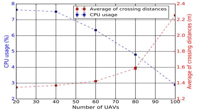
Fig. 6: CPU usage VS average of crossing distances.
