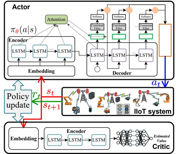
Fig. 2. The training architecture of the DRL-based JCCESP approach for multiple sensing-data-driven IIoT applications
