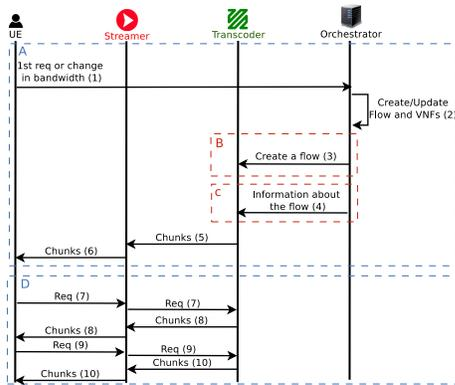
Fig. 2. Sequence diagram of the proposed solution.
