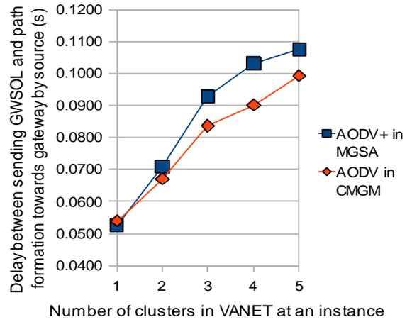
Fig. 10: Delay since the transmission of *GWSOL* till the establishment of a path towards the gateway, for varying numbers of clusters.
