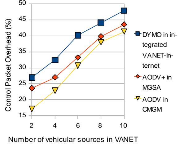
Fig. 3: Performance of the three protocols in terms of control overhead for different number of vehicular sources in VANET.
