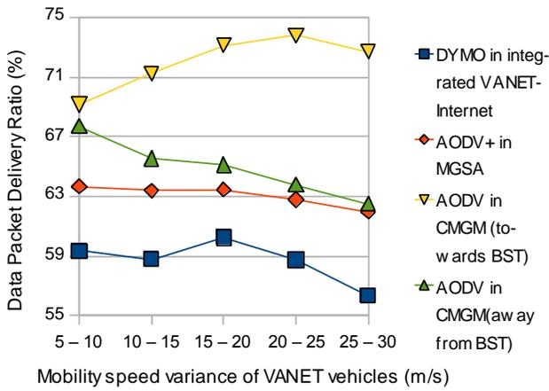
Fig. 4: Performance of the three protocols in terms of data packet delivery for different mobility speed variances.
