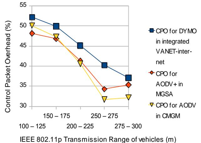
Fig. 7: CPO for different average IEEE 802.11p wireless transmission ranges.
