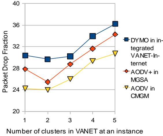
Fig. 9: Packet drop fraction for different numbers of clusters.
