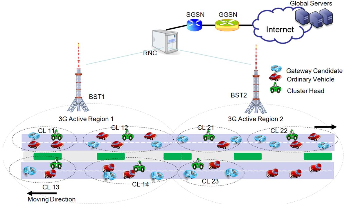
Fig. 1: Envisioned VANET – 3G integrated network architecture.
