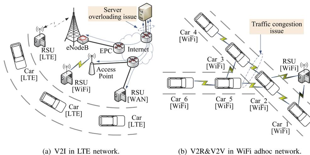
Fig. 1. Two aspects of vehicle communication.
