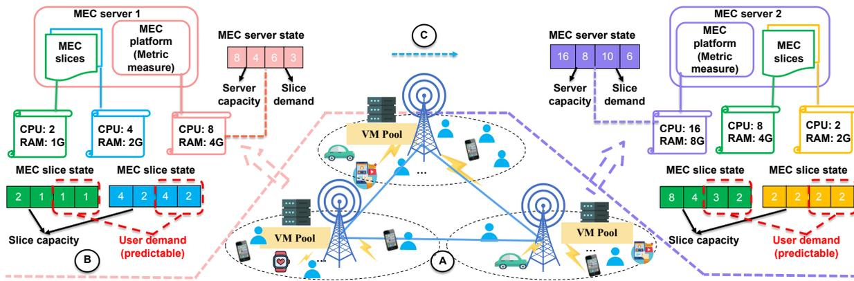
Fig. 1. Network representation for network slice mobility architecture
