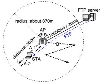
Fig. 3. Simulated network topology.
