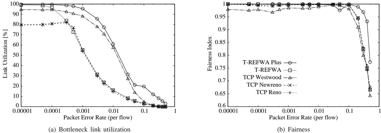
Fig. 5. Overall performance in terms of link utilization and fairness index (Flows with equal RTTs,  $N = 10$ , and possible congestion at bottleneck link  $bw = 100\text{Mbps}$ )
