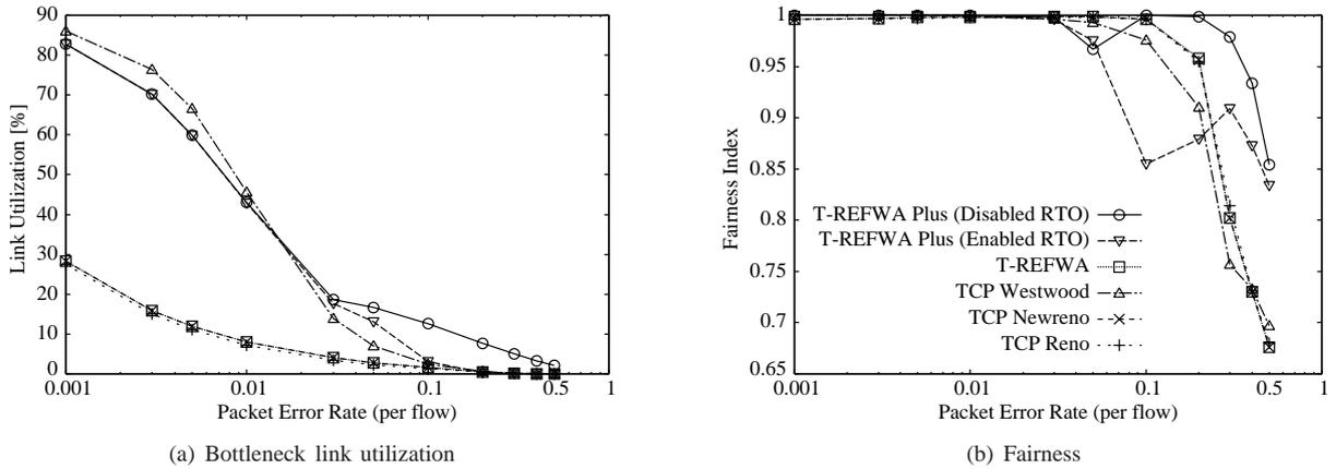
Fig. 4. Effect of the RTO backoff algorithm (Flows with equal RTTs,  $bw=200\text{Mbps}$ ,  $N=10$ )
