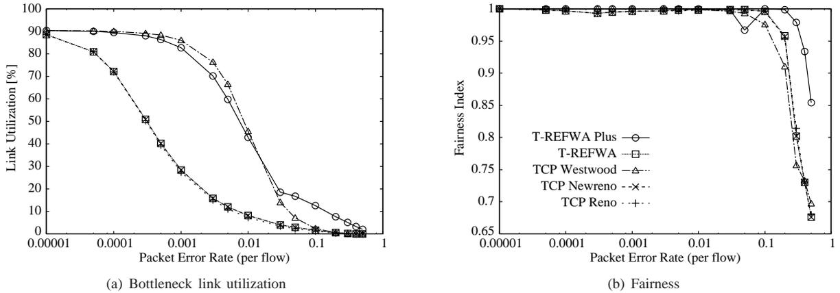
Fig. 3. System performance with no packet drops due to congestion (Flows with equal RTTs,  $bw=200\text{Mbps}$ ,  $N=10$ )
