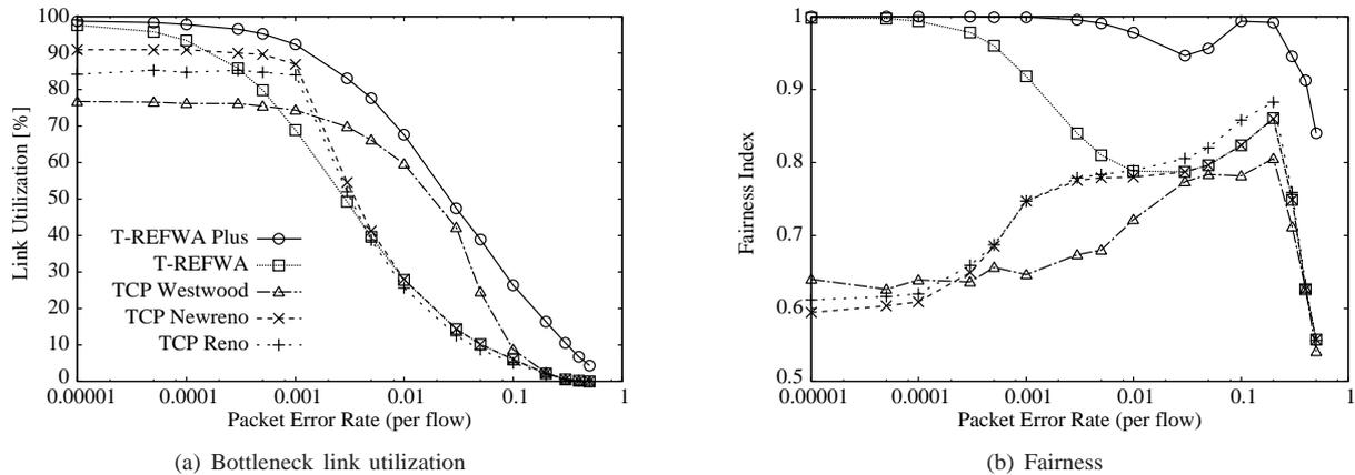
Fig. 8. Overall performance in terms of link utilization and fairness index (Flows with different RTTs,  $bw=100\text{Mbps}$ ,  $N=10$ )
