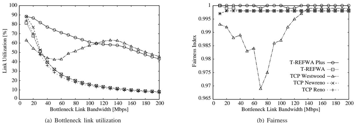
Fig. 7. System performance for different bottleneck link bandwidths (PER=0.01,  $N=10$ , flows with equal RTTs)
