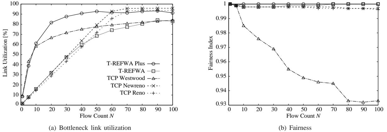
Fig. 6. System performance for different flow count (PER=0.01,  $bw=100$ Mbps, flows with equal RTTs)
